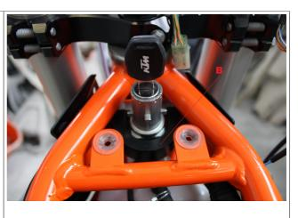
Put the U Bolt (C) on the head tube . For an easy installation of the U Bolt on the bike ,put it from the side like the picture . Once the U Bolt attach the head tube remove it slowly so the screws to be in the front and the U on the rear .
