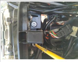
Once you remove the cables from the plastic cover you will notice that the cover have the brake lines which still hold it on its place,in order to save time just make a small cut on the plastic to remove easily the brake lines
