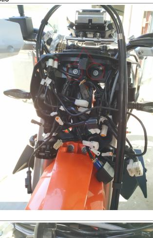
Once you remove all screws ,carefully unplug all the cables including the indicators and speedometer . Make sure you have free all the cable. ATT: There is another cable you have to un plug and its under the side cover,remove the airtubes from side panel,remove the screws from cover and locate the cable plug
