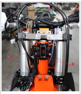
Next step is to remove from the OEM plastic the speedometer – indicators -ABS – blinkers . Do this job carefully to avoid any damages .
