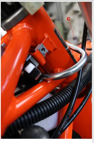
Add the main bracket (A) in the front and pass the U Bolt (C) on it .
